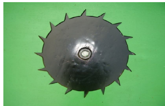
Fig. 2 Serrated blade for straw cutting
