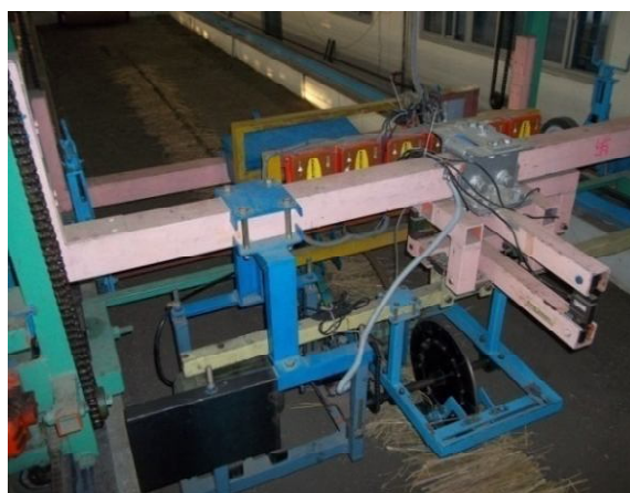
Fig. 5 Straw cutting mechanism equipped with plain blade and a pair of twin press wheels assembly
