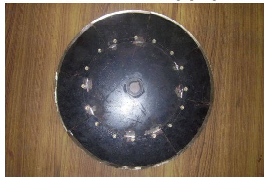
Fig. 1 Plain blade for straw cutting
